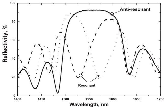
Fig. 5. Low-intensity reflectivity curves for InP SESAMs showing the difference between resonant and anti-resonant behavior.
