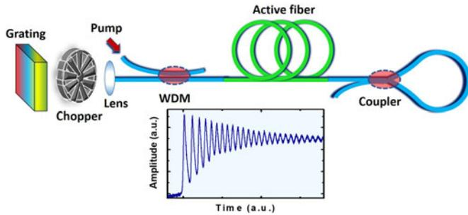
Fig. 3. The typical setup for the measurement of spectrally resolved relaxation oscillations.
