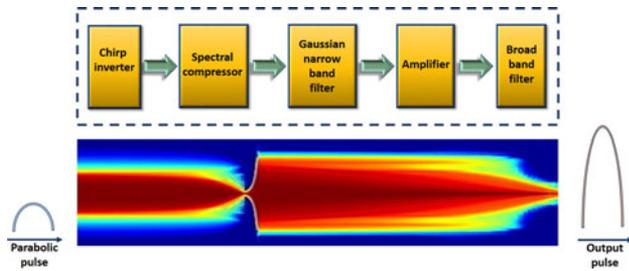
Fig. 9. An illustration of the cascade preamplifier system with spectral compression elements, and the expected evolution of the pulse spectrum.
