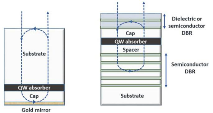
Fig. 4. General schematics of SESAMs developed at ORC. Left: SESAMs based on QWs with metal reflector and thinned substrate. Right: SESAM with monolithic DBR.
