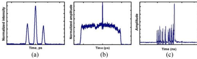
Fig. 7. Soliton complexes demonstrated in mode-locked fiber lasers: (a) auto-correlation trace of bound solitons (soliton molecules); (b) autocorrelation trace of bunch of solitons; (c) oscilloscope picture of soliton rain.
