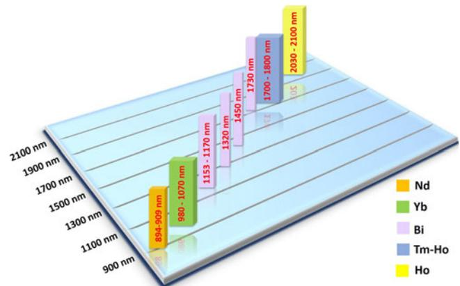
Fig. 6. The illustrative summary of new wavelengths pulse generation from mode-locked fiber laser demonstrated by Prof. Okhotnikov's group.
