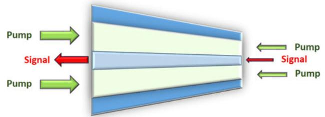
Fig. 8. An illustration of active tapered double-clad fiber.
