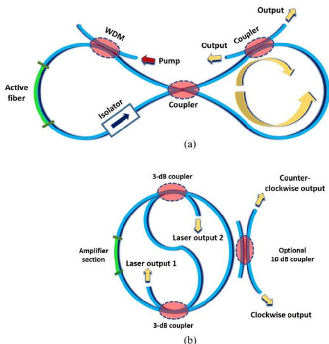
Fig. 2. The passive mode-locked fiber laser schemes. (a) Figure-of-eight-laser. (b) S-shape laser.
