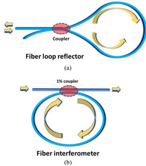
Fig. 1. The optical fiber element based on biconical fiber coupler. (a) Fiber loop reflector. (b) Fiber interferometer.
